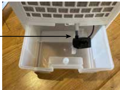
Step 3. Lift the water pump out of its compartment and let it hang freely on the hose.
